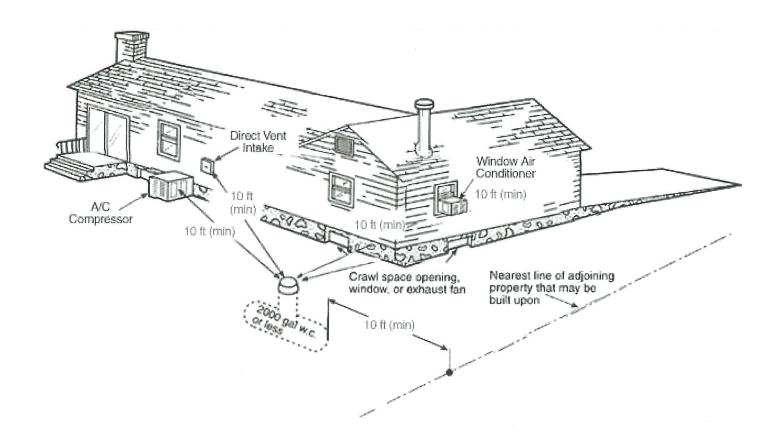
Note: When the cylinder is filled on site from a bulk truck, the filling connection valve and vent valve must be at least 10 feet from any exterior source of ignition, opening into direct-vent appliances, or mechanical ventilation intakes.
