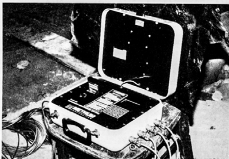
Figure 20. Portable monitors used to record temperature and humidity conditions in historic buildings during mothballing can help identify ventilation needs. This data can be downloaded directly into a lap top computer on site. These monitors are especially helpful over the long term for buildings with significant historic interiors or which are remaining furnished. If interiors are remaining damp or humid, additional ventilation should be added or the source of moisture controlled.
