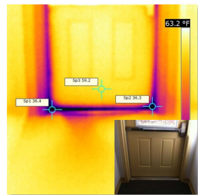
Figure 9: Air Leakage at Door Frame
